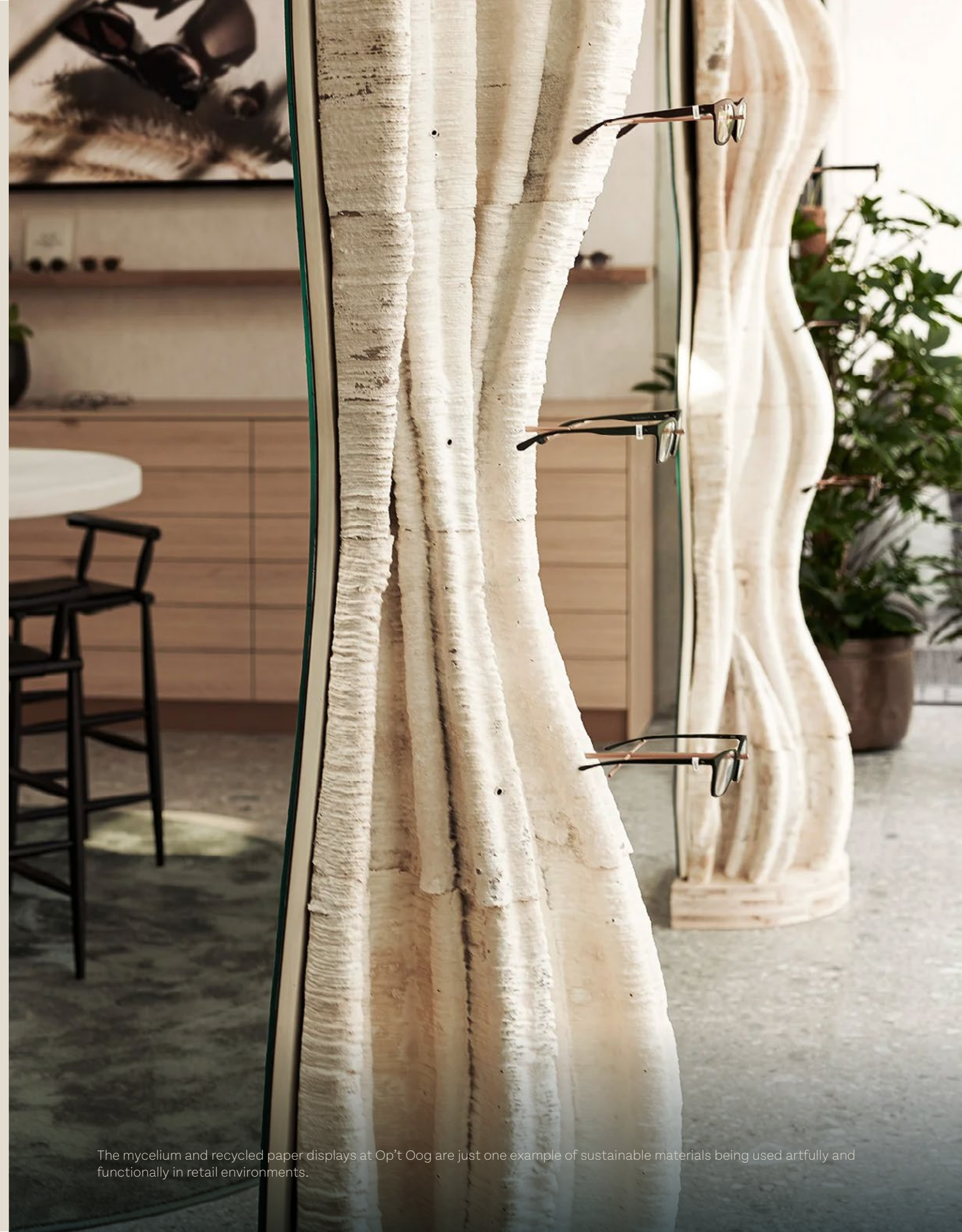
A 3D printer constructs columns from recycled paper coffee cups, which becomes the armature for mycelium to grow and create the final product.
