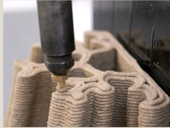
A 3D printer constructs columns from recycled paper coffee cups, which becomes the armature for mycelium to grow and create the final product.
